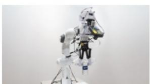
This novel robotic system developed by National University of Singapore researchers comprises an artificial brain system that mimics biological neural networks, which can be run on a power-efficient neuromorphic processor such as Intel's Loihi chip, and is integrated with artificial skin and vision sensors. (Credit: National University of Singapore) » Click for full image
