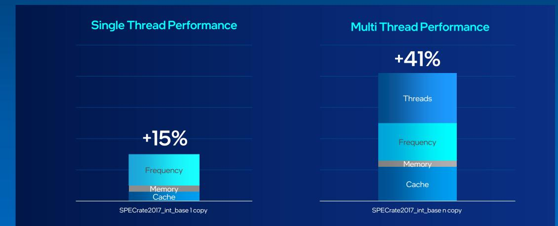
Source Intel: As estimated by measurements made using SPECint\_rate\_base2017\_IC2022.1 (1-copy & n-copy) using Intel validation Platforms comparing Core i9 13900K versus Corei9 12900K Frequency includes enhancements to the CPU and the Fabric
