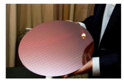
7th Gen Intel Core processors are manufactured on silicon wafers at Intel
