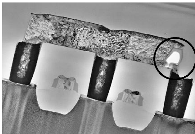
Figure 12: Example of a Metal 1 void failure due to pullback, before process optimization
