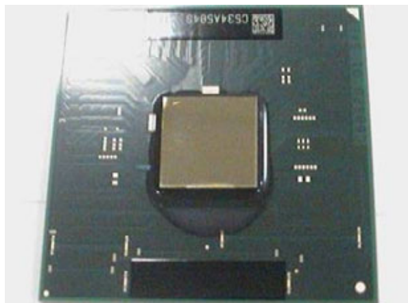
Figure 13: Example of underfill spread on a flip-chip CPU package
