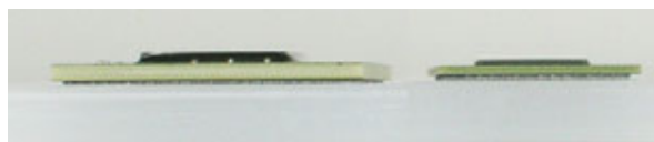
Figure 18: Comparison of a standard package z-height with a thin core-thin die package
