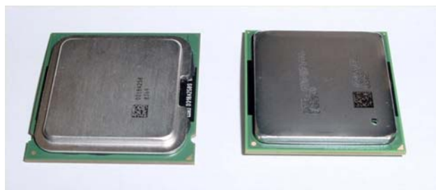
Figure 3: LGA775 and mPGA478 packages
