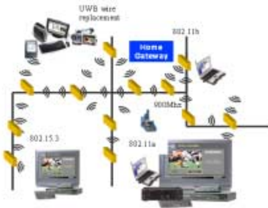
Figure 3: A multi-hop backbone must interface with multiple PHY/MAC layers in the home
