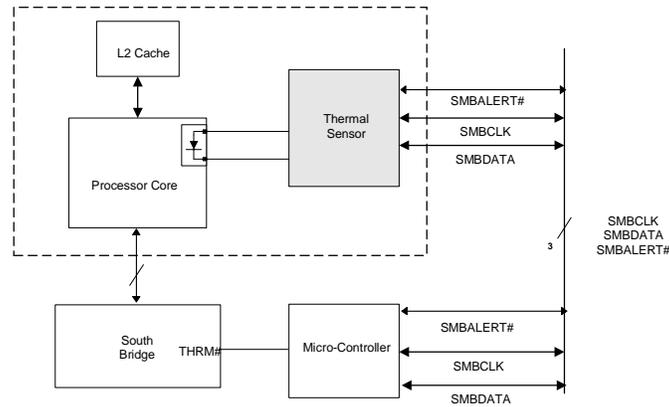
**Figure 1. An Example of Microcontroller Driven Thermal Management**
