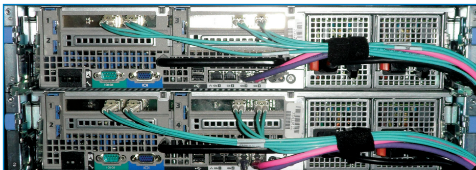
Figure 2. Simplified server connectivity using 10 Gigabit Ethernet.
