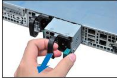
Figure 46. Power Module Removal
