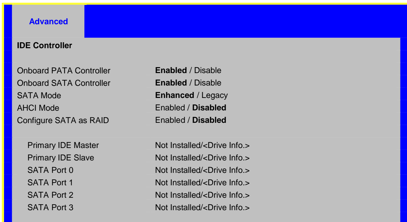
Figure 10. Setup Utility — SATA Controller Configuration Screen Display
