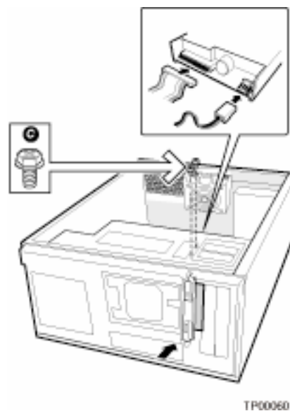
Figure 8: Drive Bay Locations for Server Chassis SC5275-E
