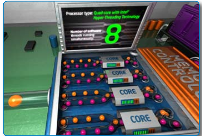
Intel® Hyper-Threading Technology makes a return appearance, accelerating applications by handling up to eight threads on four cores.
