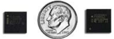
solutions which, when combined, deliver a complete WiMAX connectivity solution for notebooks and other devices. Intel WiMAX silicon solutions support very small form factors while minimizing design overhead and power consumption, as well as improving performance.
