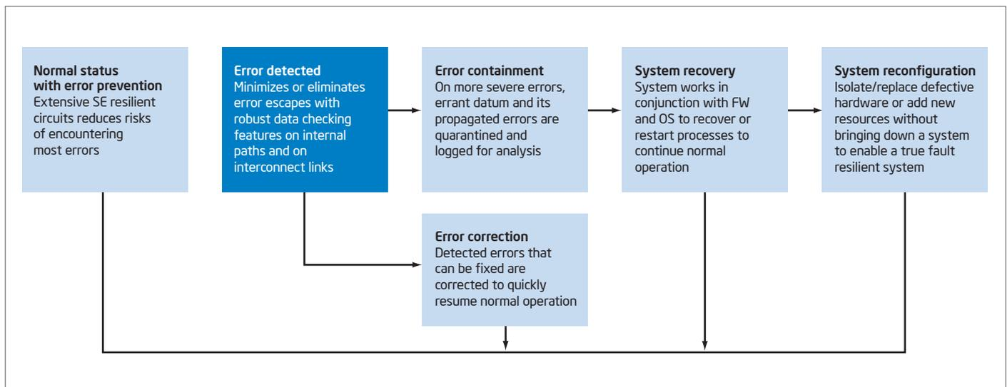
**Figure 4.** The extensive error detection and correction mechanisms in the Intel® Itanium® processor 9300 series, combined with its Advanced Machine Check Architecture, enable comprehensive error management to optimize both system uptime and data integrity.
