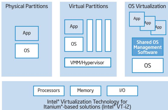
**Figure 5.** Itanium-based servers support multiple partitioning options to enhance IT flexibility and resource utilization. Advancements in the Intel® Itanium® processor 9300 series – such as Intel® VT-i2 and native support for dynamic partitioning and dynamic resource allocation – deliver enhanced support to provide organizations with greater flexibility, better performance and more consistent solutions across vendor implementations.
