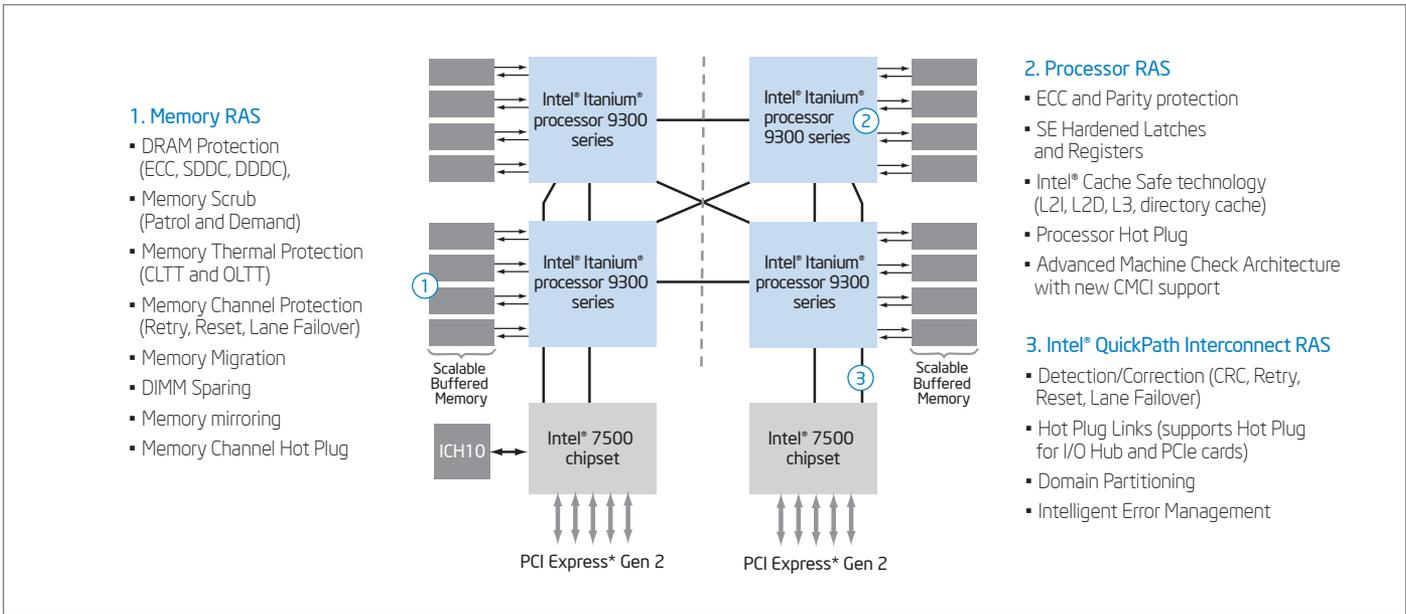
**Figure 2.** The Intel® Itanium® processor 9300 series provides comprehensive support for error avoidance, detection, correction, containment and reporting across all major structures.
