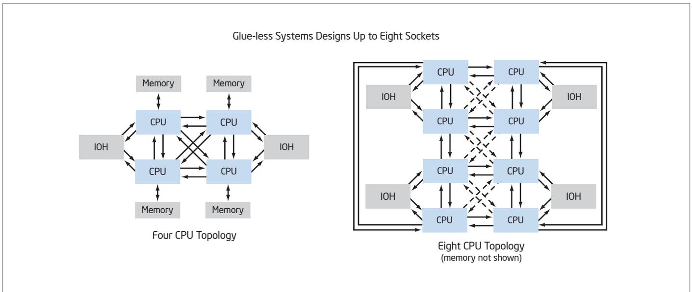
**Figure 1.** The quad-core Intel® Itanium® processor supports up to eight-socket glueless system designs. Larger symmetric multiprocessing (SMP) systems are built using node controllers designed by the individual system vendors.
