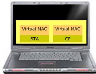
Figure 3: Intel MWT virtual radios enable a notebook to support concurrent WLAN and Wi-Fi PAN connectivity
