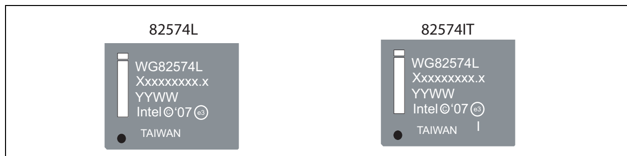
Figure 2. Production Top Marking Example With Identifying Marks
