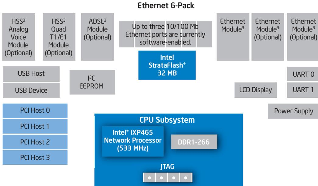
Figure 2: Intel® IXP465 Development Platform Board Diagram
