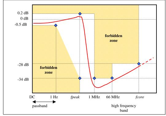
Figure 3. Phase Lock Loop (PLL) Filter Requirements
