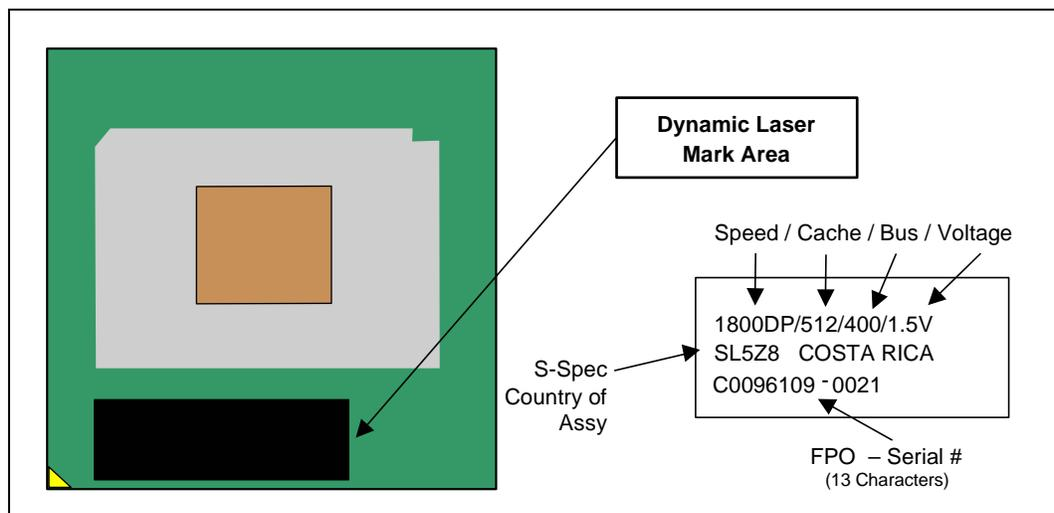
Figure 5. Example of Production Mark – Top View
