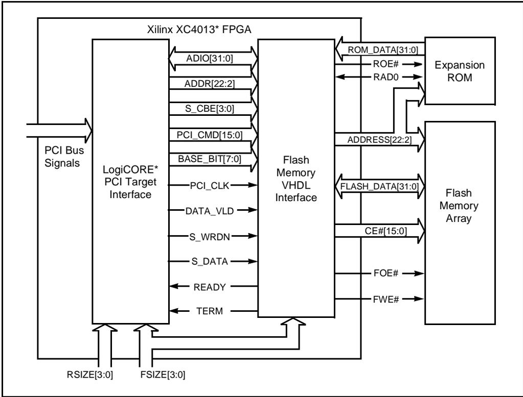
Figure 5. VHDL Code Block Diagram
