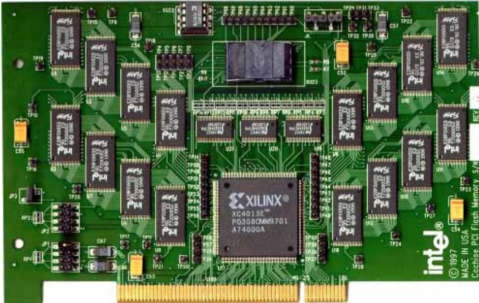
Figure 1. Flash Memory PCI Add-In Card
