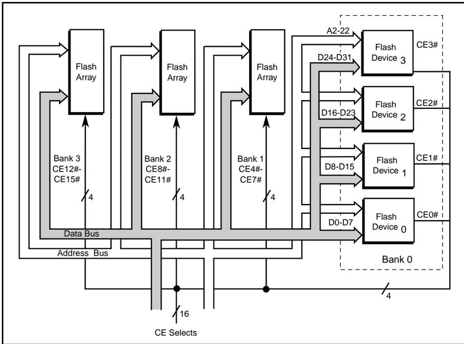
Figure 3. Flash Memory Array Block Diagram
