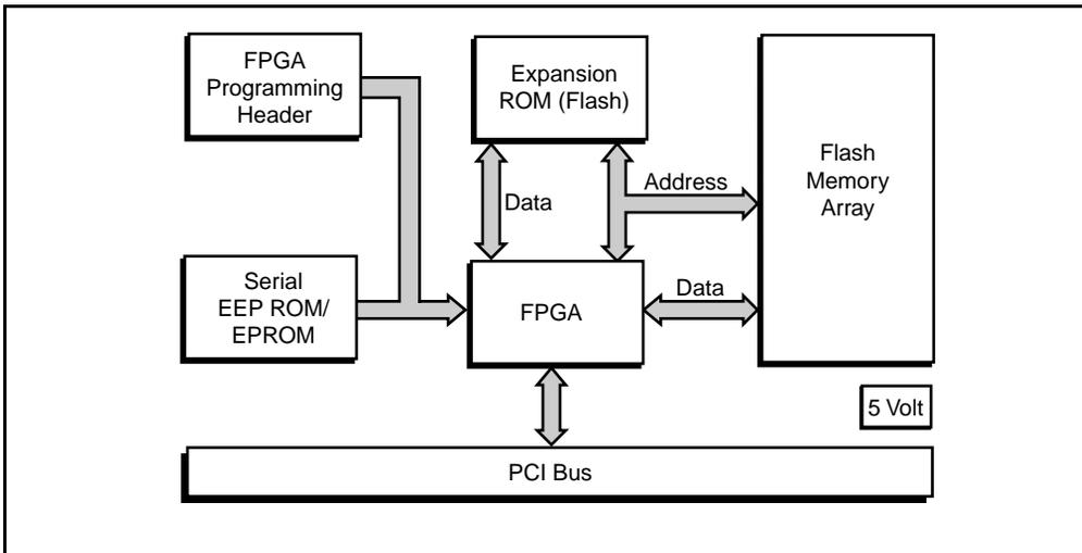
Figure 2. Flash Memory PCI Add-In Card Block Diagram
