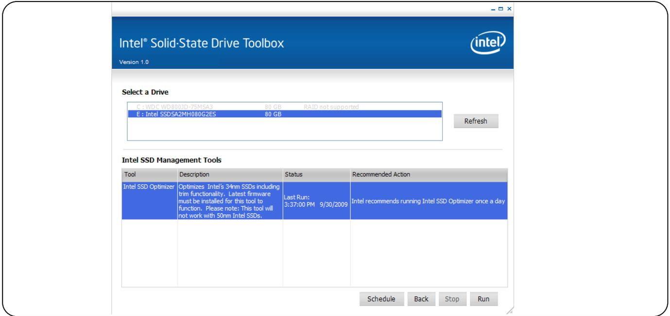
Figure 5. Intel SSD Management Tools screen showing Intel® SSD Optimizer function
