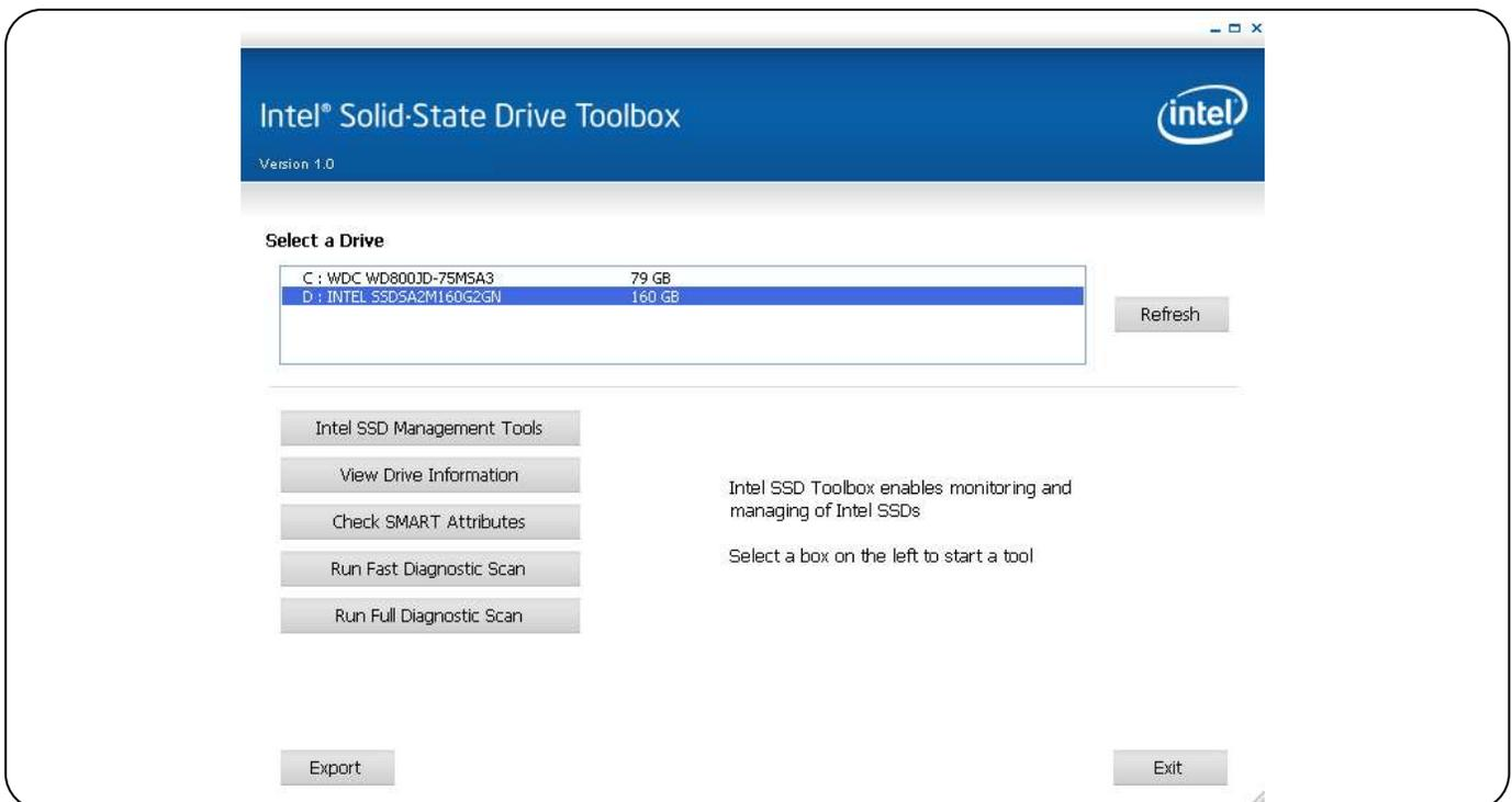
**Figure 4.** Intel® Solid-State Drive Toolbox home screen
